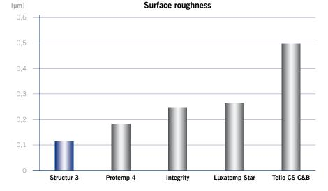
The chart shows Structur 3 as having the lowest level of surface roughness after having been wiped with a cloth soaked in alcohol.
